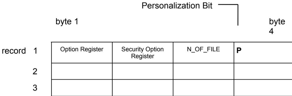
The first three bytes of the first record of the Personalization File are used to set certain parameters and to enable/disable optional features of the card operating system:
