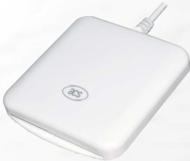
**The ACR38 is the flagship product of ACS. It is a powerful and reliable smart card reader that supports smart cards conforming to ISO 7816.**
