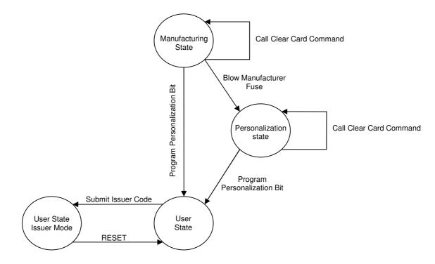
The actual chip life cycle state is determined by the card operating system immediately after a reset. The life cycle state does not change during the operation of the card. Clear card command can be issued in the personalization state and manufacture state to clear the card of all data except the manufacturer data and IC code. However, this command will not be able to be used after user state.
